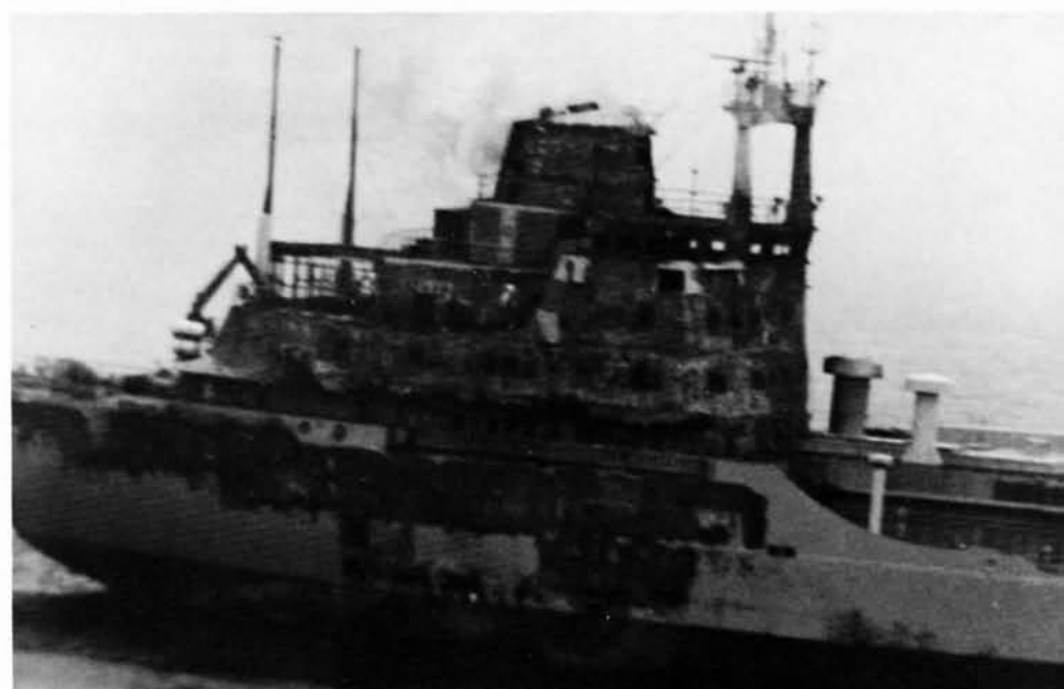
Figure 2. Bridge area of MV Essi Silje on fire. Note hot spots (dark patches) appearing on hull.
