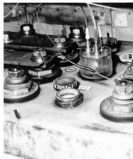
Fig. 4. A battery probe installed in a cell.
