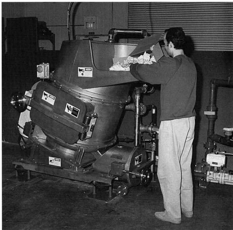
A pre-production prototype of a shipboard solid-waste pulper is put through its paces at the U.S. Naval Research Laboratory in Annapolis, Maryland.
