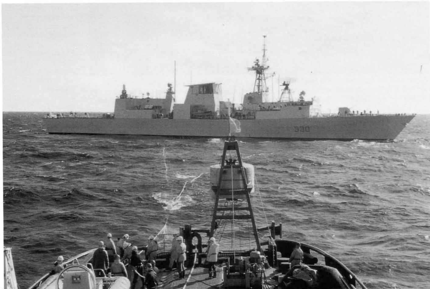
Fig. 5. Final preparations: HMCS Halifax positions herself across Riverton's stern and passes lines to deploy the bridle assembly. (CFB Halifax Base Photo)
