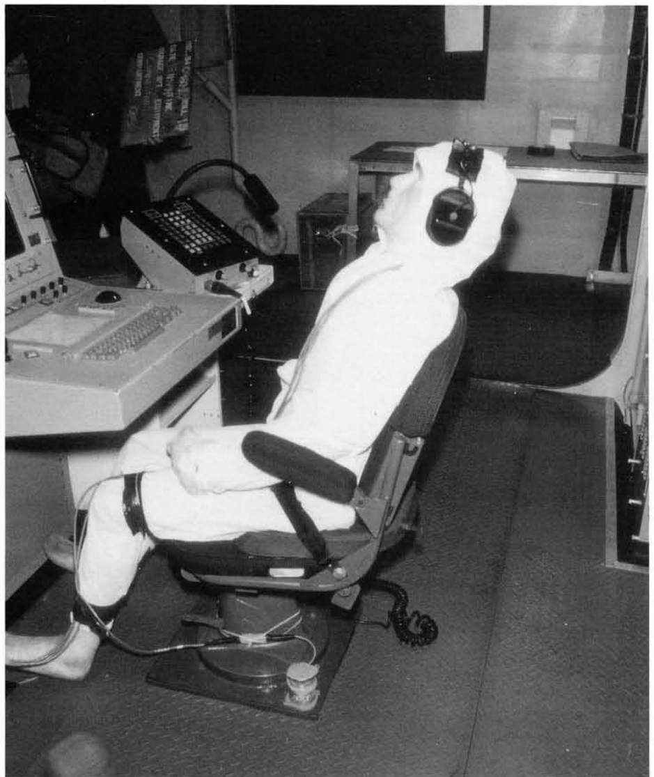
Veterans of numerous personnel vulnerability investigations, mannequins such as this one in Halifax's operations room were fitted with triaxial accelerometers to measure shock response. The gauge on the deck below the seat monitored the shock input. (NETE photo by George Csukly)
