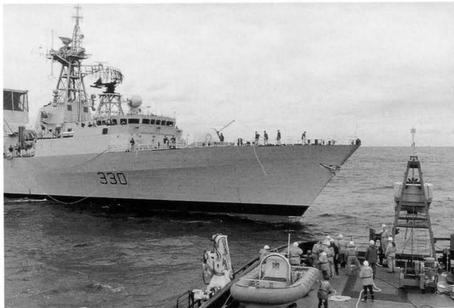
HMCS Halifax passes lines to Riverton in preparation for a shot. The charge float is visible on the A-frame, but the charge itself has already been armed and lowered to depth. (CFB Halifax photo by MCpl M. Ray)
