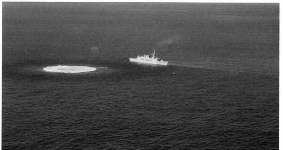
Shot 3: The big one. This series of photos taken from one of the helicopters shows the effects of the initial shock wave reaching the surface ( top ), the formation of the plume ( centre ), and the formation of a three-metre surface wave. ( CFB Halifax photos )
