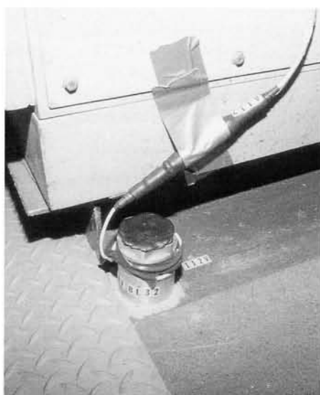
One of the many accelerometers fixed throughout HMCS Halifax to capture data during the shock trial. (CFB Halifax photo by Cpl. R. Duguay)
