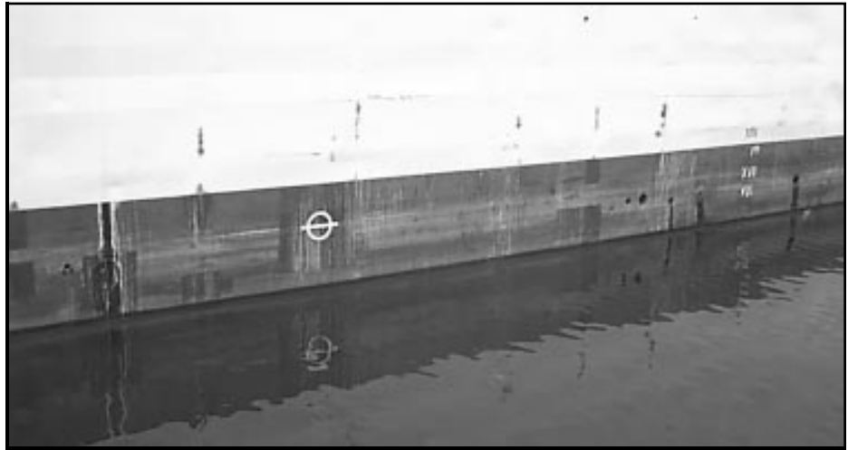
Samuel Plimsoll’s load line mark — an important addition to the weight-critical Iroquois class.
