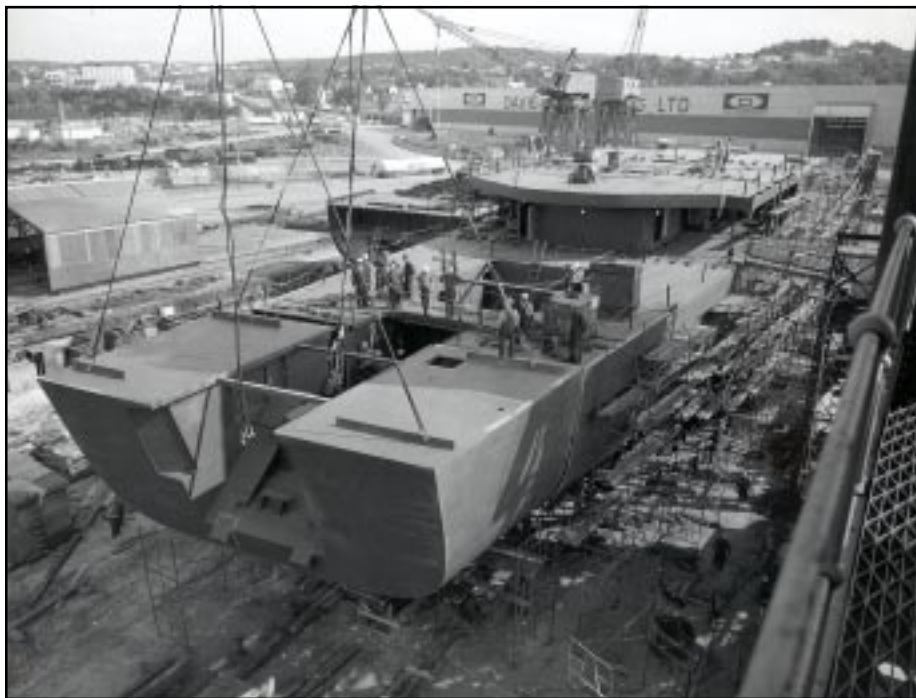
Job H-670 (HMCS Athabaskan ) under construction at Davie Shipbuilding Ltd., Lauzon, Québec in July 1970. (Davie Shipbuilding Ltd. photo)
