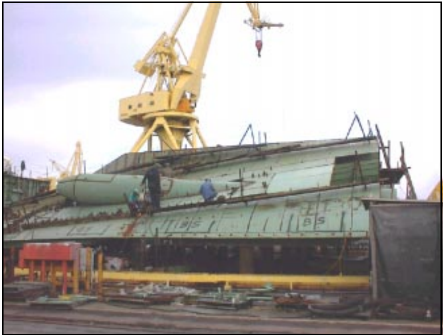
In many ways the USN DDG-51 build program was reminiscent of our own patrol frigate program. Downhand construction and extensive pre-outfitting were very much the order of the day. (Photo by Robert Cole, courtesy Ingalls Shipbuilding)
