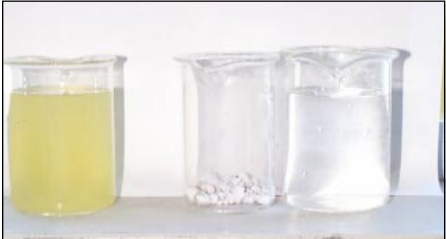
Fig. 8. Waste before treatment (left) and after (two beakers at right). (DND photo.)
