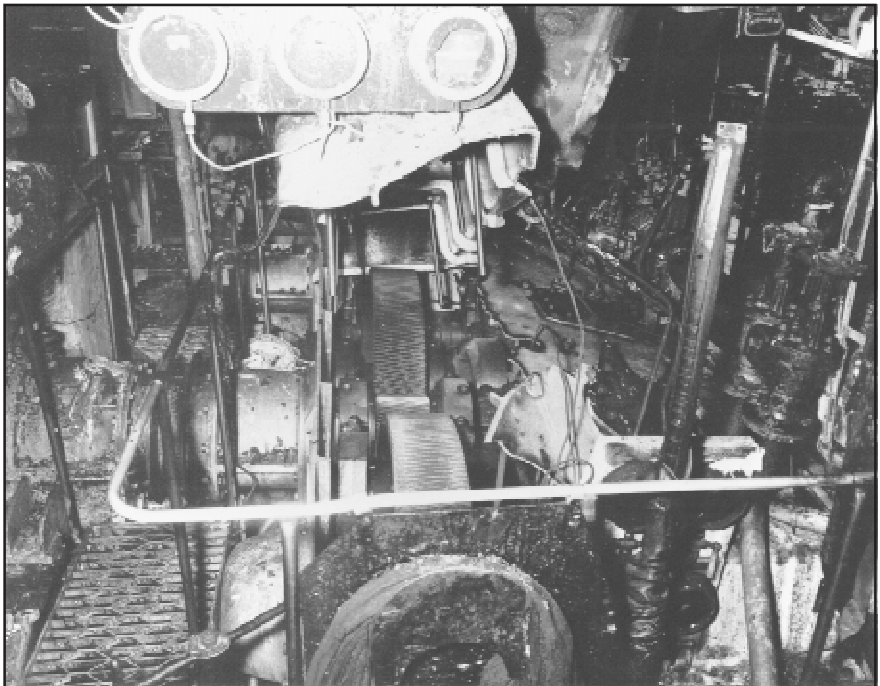
Fig. 1. The blackened engine room of HMCS Kootenay in the aftermath of a devastating gearbox explosion and fire bears dark witness to the horrific events of October 23, 1969. An improperly assembled forward pinion journal bearing lay at the heart of what should have been an avoidable tragedy. (All photographs property of DND)
