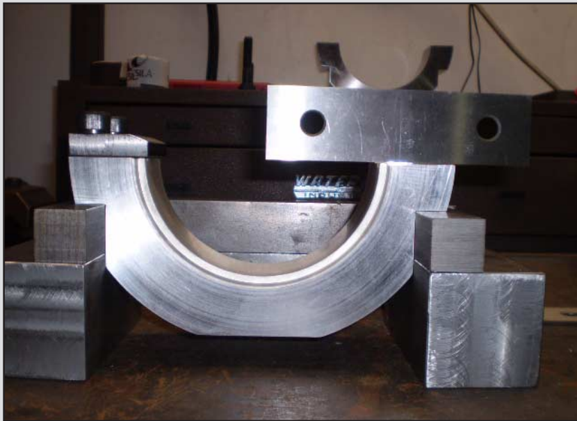
Fig. 6. Wartsila Canada’s Halifax facility manufactured this highly accurate jig to measure nip lengths of the conrod bearings.
