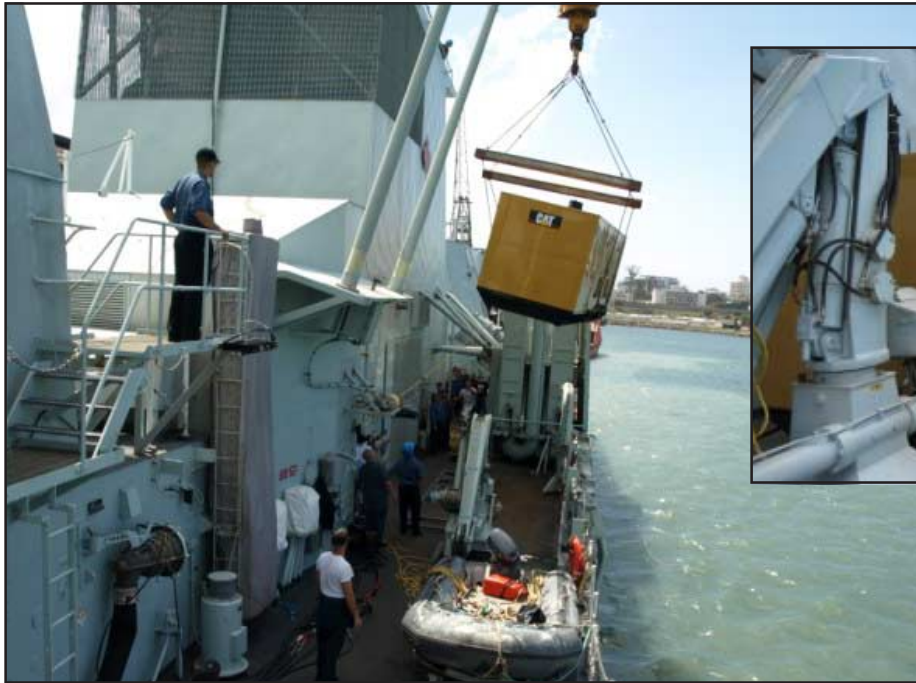
A tight fit on the port side. A less-than-ideal sling mechanism and minimal clearances on the superstructure complicated the installation.
