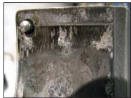
Fig. 2. The conrods showed a high degree of fretting and significant levels of material transfer between the big-end cap housing and the bearing.
