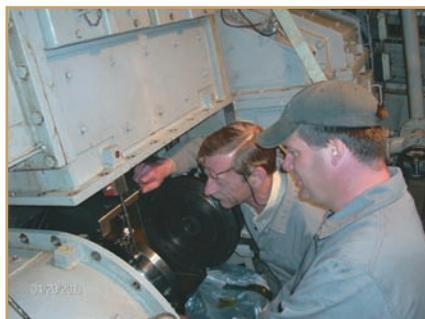
Step 5. FMFCS mechanical fitter Jim Rankin (foreground) and author Bob Steeb check the flange run-out readings.
