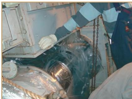
Step 2. The gearcase section is removed.
