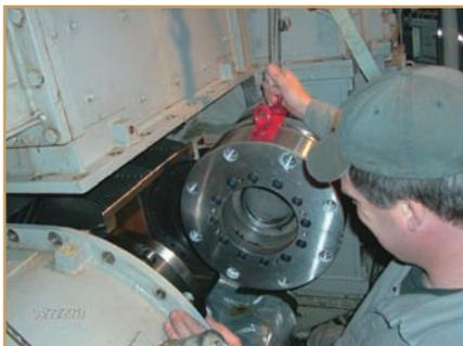
Step 4. The exposed clutch is lifted out using a single transport bracket.
