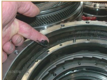
Step 12. A significant build-up of sludge in some areas indicated where contaminants had accumulated over the life of the clutch, and might also have been related to the noise problem in the clutch.
