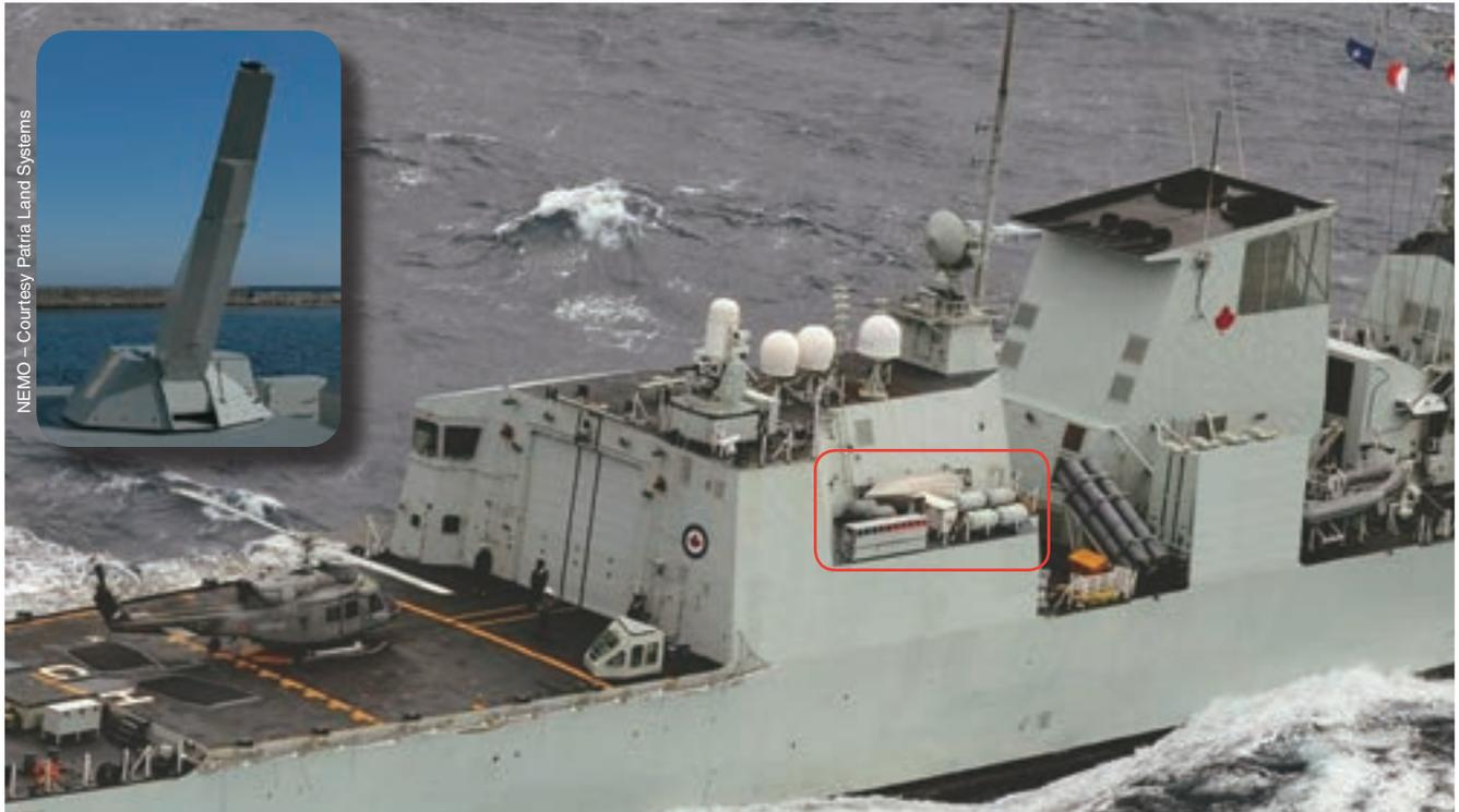
The author's proposed site for a precision-guided weapon mount on board some *Halifax*-class frigates is on the starboard mezzanine deck between the hangar and the funnel.
