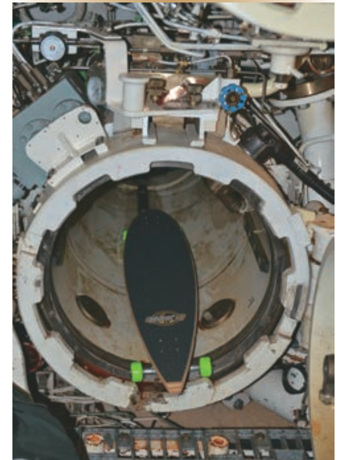
This 'Submarine Kinetic Access Tube Examination (SKATE)' board was very useful as a mechanic's dolly for torpedo tube inspections.
