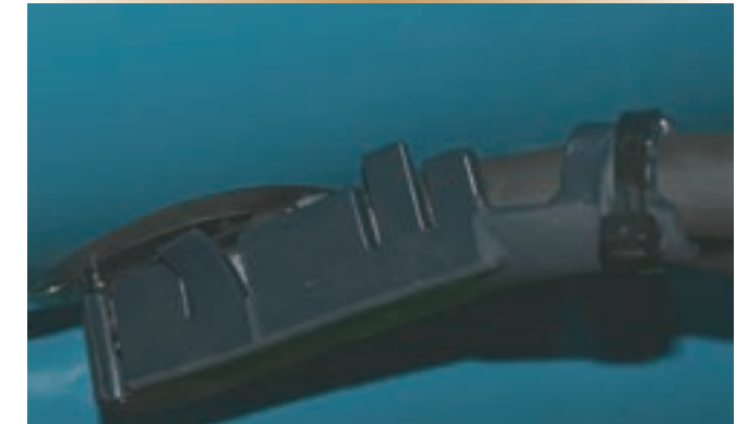
This high-density rubber 'boot' was designed by the U.S. Naval Undersea Warfare Center to protect the A-Cable ends inside the torpedo tube during discharge.
