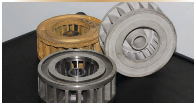
Figure 2 – Three versions of a NASH compressor impeller: Front left is the laser additive manufacturing replica, while behind it is the brass original part. On the right is a plastic replica produced using 3D printing.
