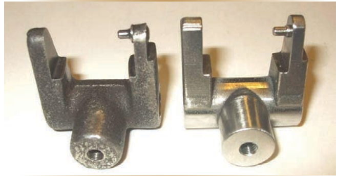
Figure 1 – This fuel flow meter component (original is on the left) was reproduced at right using additive manufacturing. The part has been in service for more than two years without failure.
