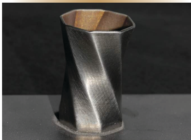
Figure 3 – This R&D test piece was created to demonstrate multiple-axis additive manufacturing capabilities which cannot be produced using computer numerical control milling equipment.
