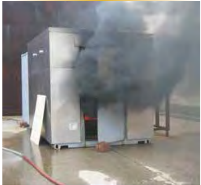
Figure 3 – An insulated burn room constructed inside this ISO shipping container allowed for a good simulation of a fire in a small machinery space, and the measured effectiveness of a small aerosol extinguisher (shown) in that space.
