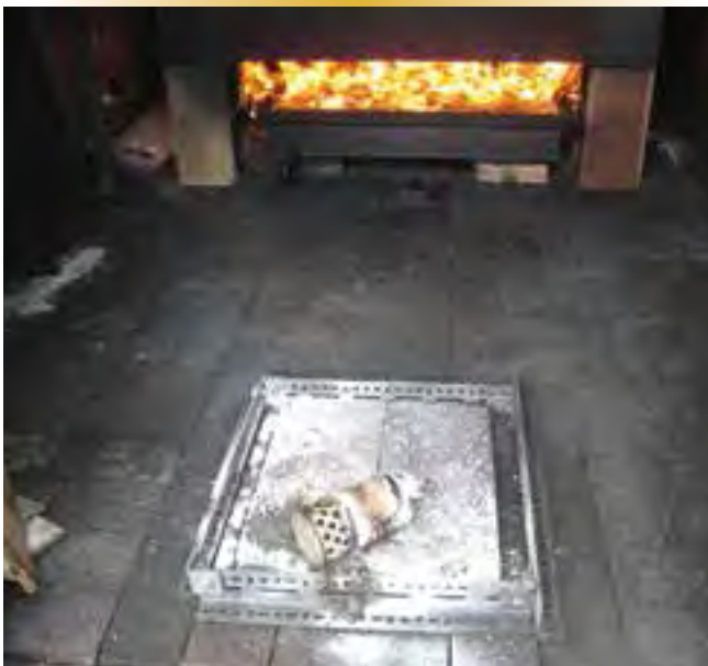
Figure 3 – An insulated burn room constructed inside this ISO shipping container allowed for a good simulation of a fire in a small machinery space, and the measured effectiveness of a small aerosol extinguisher (shown) in that space.
