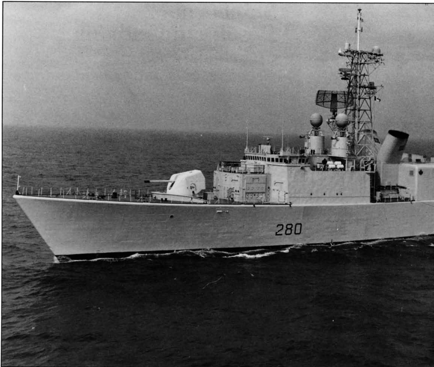
Gas - turbine ships must produce two tons of fresh water each hour to meet machinery and domestic requirements.(HMCS Iroquois)
