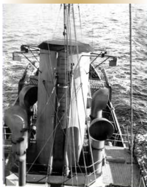
HMCS Kamloops with diffused lighting camouflage fittings on struts around the funnel, September 1941.
