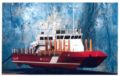
The vessel has provision for the deployment of an additional sonar transducer from the crossbridge and is equipped to support secondary roles such as; Navigation Aids Maintenance, Search and Rescue and Pollution Cleanup.
