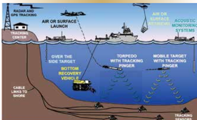
Geometry schematic of a typical 3-D underwater tracking range.
