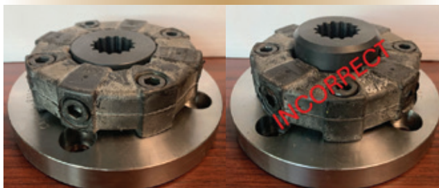
Correct vs incorrect assembled coupling
