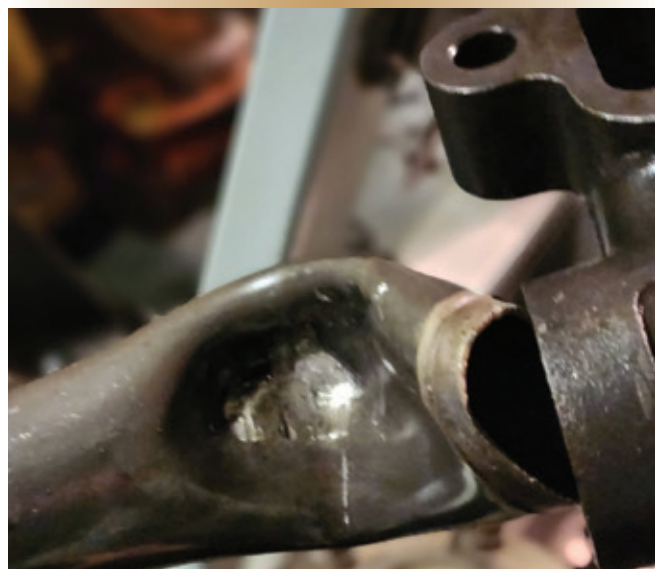
Damage to oil pump discharge
