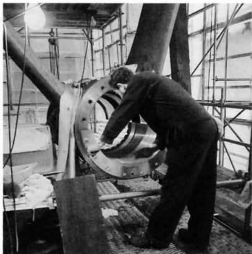
Final check on the port main A-bracket bearing.
