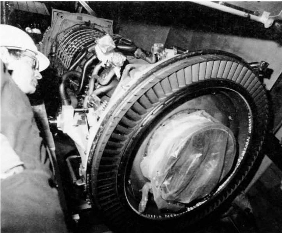
Fig. 2 A good view of the turbine end of the gas generator, now clear of the enclosure plenum. The #6 bearing has been protected by a sheet of plastic as it is the most vulnerable part of the gas generator when it is exposed like this.
