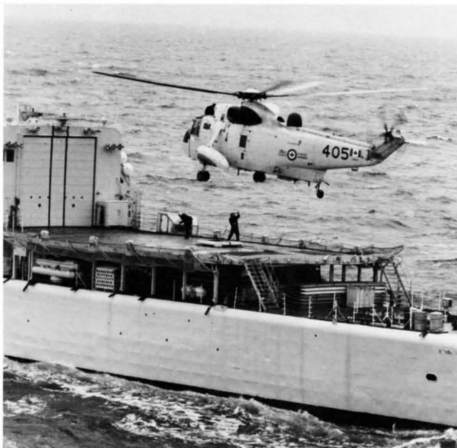
Figure 5. RAST MK III eliminates the requirement for flight-deck personnel during recovery/launching operations. (DND photo)
