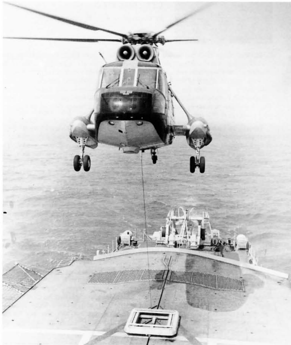
Figure 1. "Flying the wire," necessary with the HHRSD, RAST MK I and CPF RAST systems, will become a thing of the past with the "wireless" RAST MK III. (DND photo)
