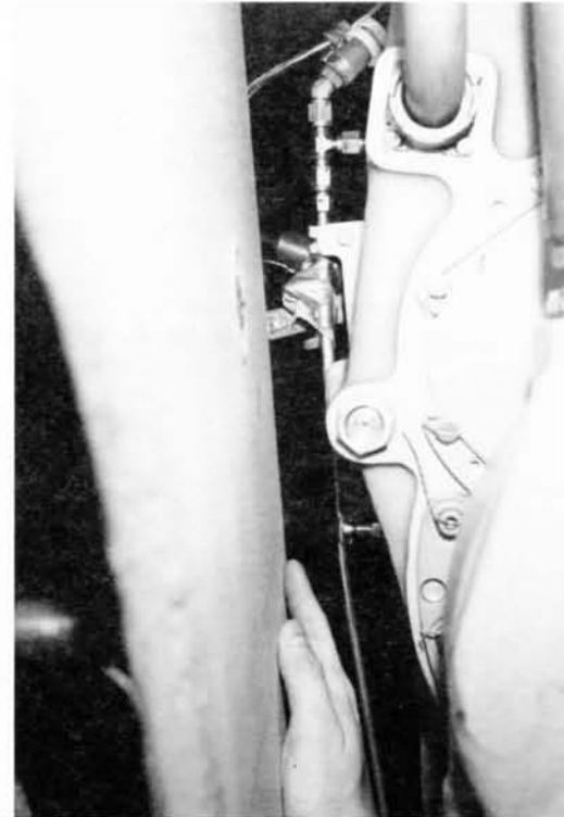
Fig. 3 Minimal clearances like this can be easily checked prior to removal with a representative-sized jig.
