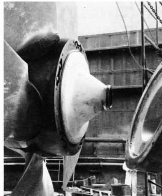
Figure 2. With the foam-filled fairing cone pulled away (right), the white tallow pressed against the hub is revealed. This part of the underwater operation required careful planning to prevent the buoyant cone from floating away out of control.
