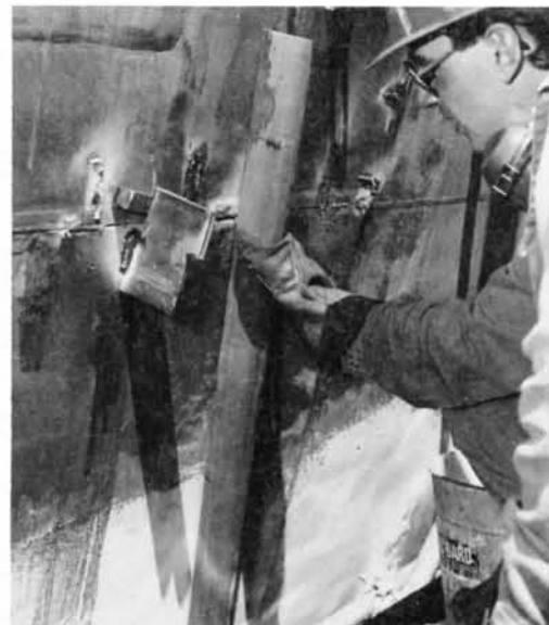
Fig. 7. Fairing the hull using L-brackets.
