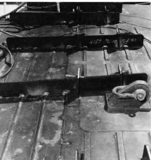
Fig. 8. Preparing for final welding, strongbacks are welded and wedged into slotted brackets on either side of the weld-line to prevent distortion.
