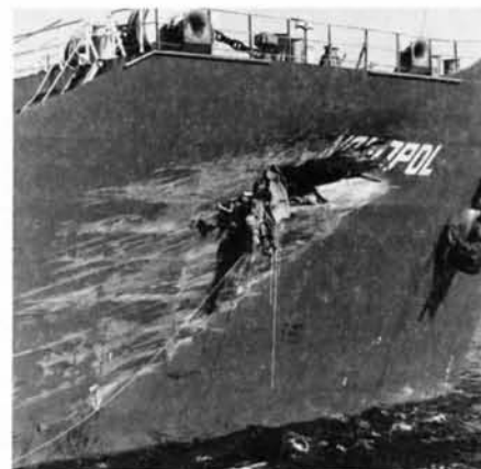
Fig. 1. Bow section of the MV Nordpol following the collision. A crumpled piece of Kootenay's steel plating protrudes from the gash.
