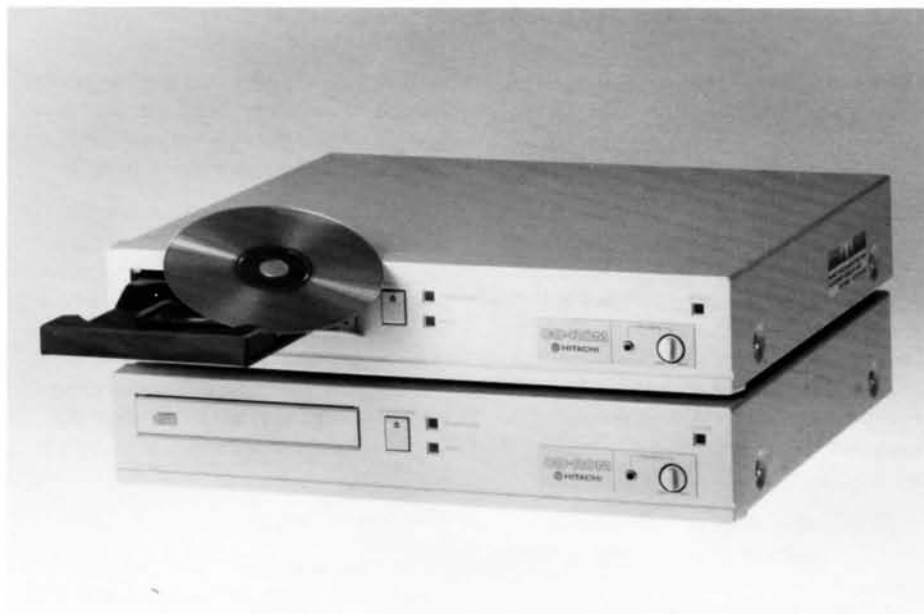
CD-ROM: the way of the future for shipboard information management. These two CD-ROM drives were installed in HMCS Huron in 1991 for the shipboard trial of a prototype electronic version of the CF Equipment Support List. (NETE photo by George Csukly)
