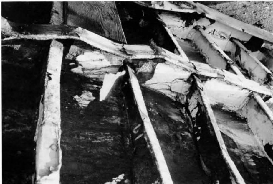
Fig. 1. The extremely corroded structure found in this ship's machinery space is blunt testimony of inadequate survey and repair.
