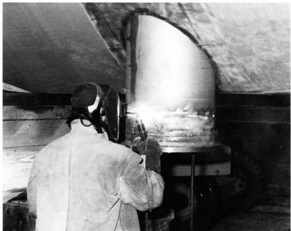
Fig. 3. The sea tube of the CTS-36 system on Restigouche . (Base Photo Esquimalt)
