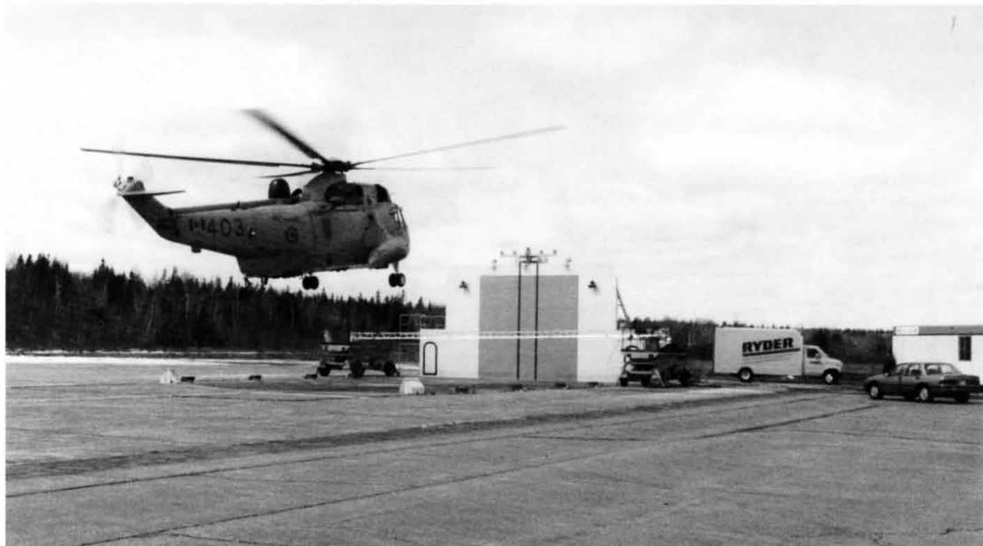
In preparation for shore-based testing of the RAST Mk III Helo Position Sensing Equipment and Pilot Cues Controller at CFB Shearwater, a mock-up 205-class hangar and flight-deck are subjected to downwash from a Sea King helicopter. (NETE photo by Peter Michetti)
