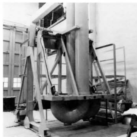
This Mk 48 GMVLS shipboard mounting interface was installed as part of the new land-based test site in Halifax. (Photo by Base Photo Halifax)
