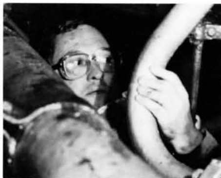
Fig. 2. There is no automated diagnostic system for identifying structural faults. Careful area examinations and experience in knowing what to look for are the keys to successful hull health monitoring. (Photo: Base Photo Esquimalt)
