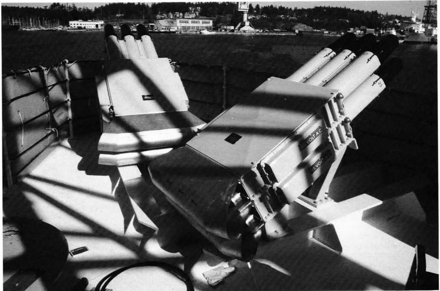
These Shield ECM launchers make an interesting study in shadows on Restigouche's starboard gun-direction platform extension. Installed for Op Friction II, the Shield system will cover the ship against missile threats during Operation Barrier. Radar absorbent padding has been placed around the stanchions and guardrails. (Photo by LCdr R.B. Houseman)
