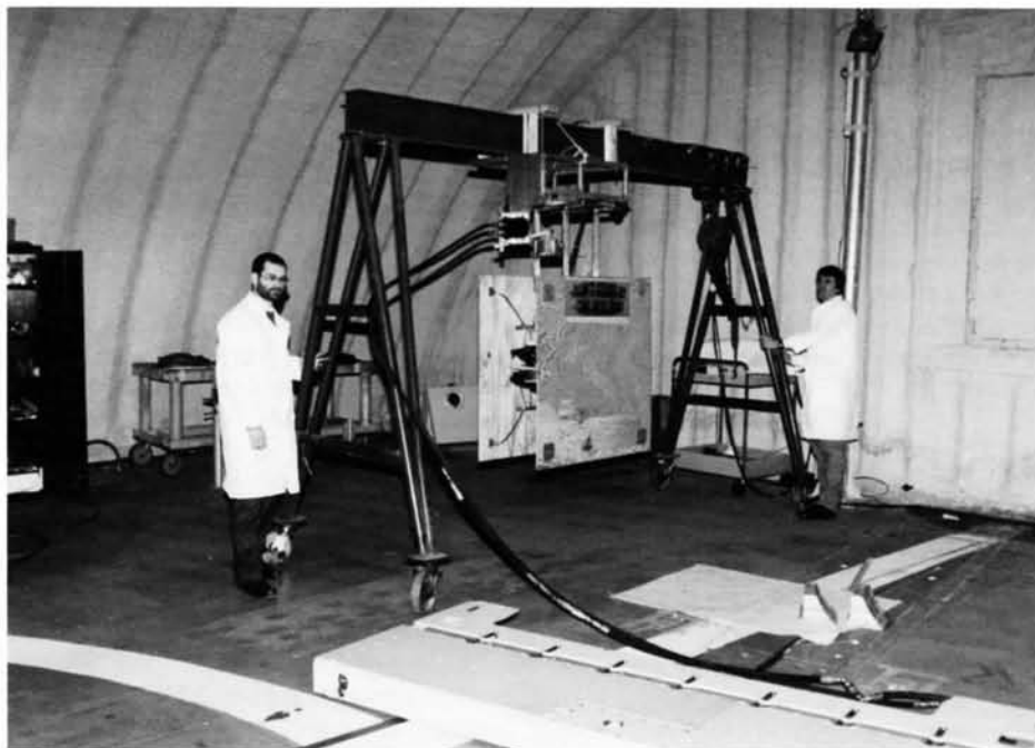
Indal technicians manoeuvre a simulated helicopter airframe to demonstrate the integration of hardware/software components of the RAST Mk III helo handling system. The Rapid Securing Device is visible in the foreground, while in the background the infra-red sensing camera can be seen just to the left of the boards suspending the beacon array. (Photo courtesy of Indal Technologies Inc.)
