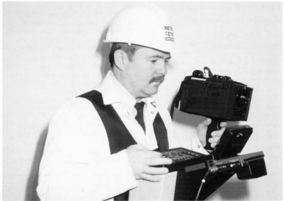
The Inframetrics thermal imaging system: note the portability of the system with its hand-held camera and vest-mounted control unit. The Sony 8-mm Video Walkman on top of the control unit allows thermal images to be displayed and recorded.
