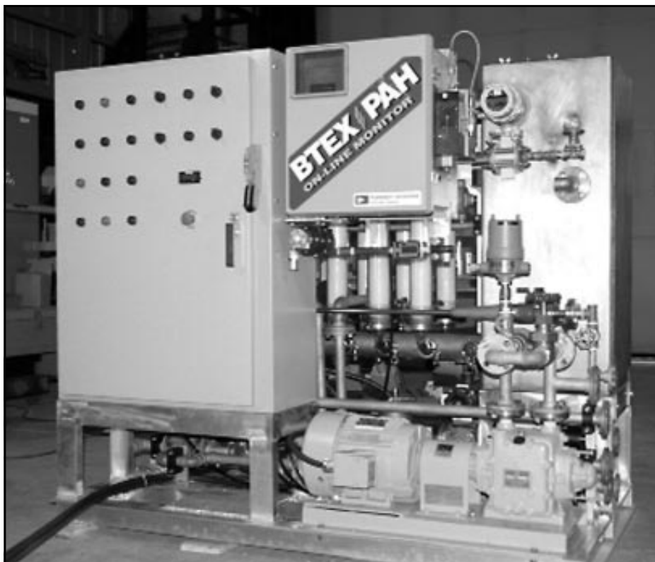
The new Hydromem™ oil/water separator system destined for shipboard installation this fall will fit in the same footprint as existing units. Some of the spindle-like ultrafiltration membranes are visible to the left of the tall effluent collection tank at right. The PLC controller is on the left. (Photo courtesy Water Technology International Corporation.)
