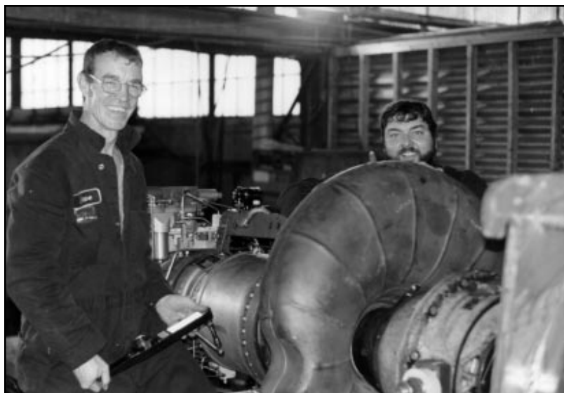
Solar gas turbines being prepared for installation: Two large access ports were cut into the side of the ship at the AMR to accept the machinery.
