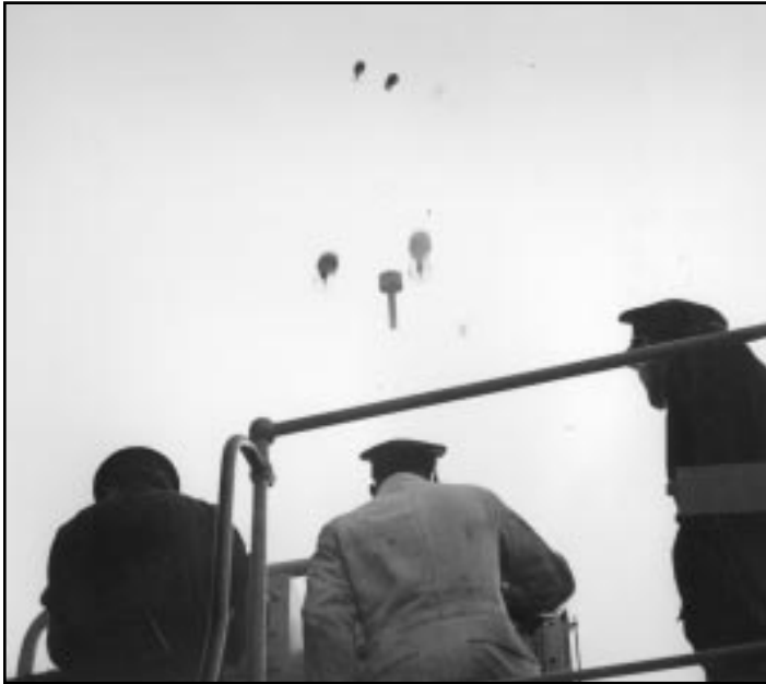
Bombs away! The Hedgehog threw its twenty-four bombs ahead of the ship to land in a circle whose diameter was about two-thirds the length of the U-boat. They fired on contact only. (National Archives of Canada photo R-707, courtesy the Directorate of History and Heritage)
