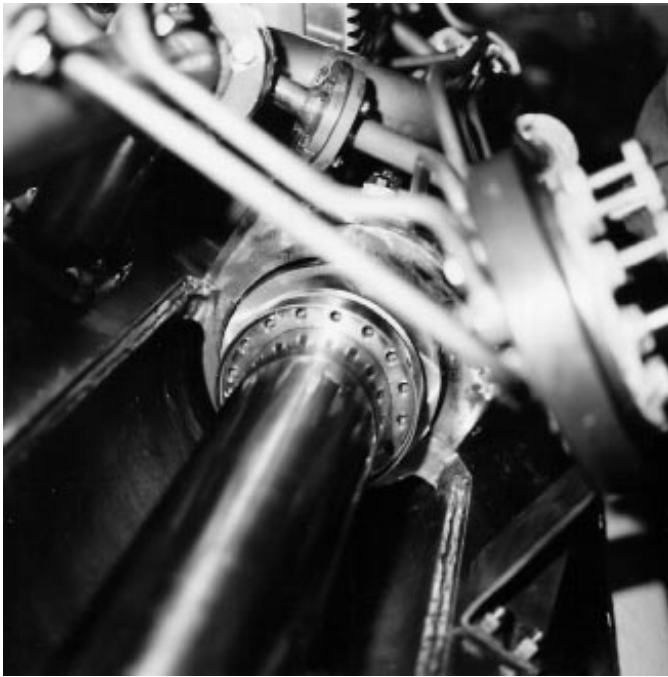
Fig. 7. The after flange (centre) — minus its bolt heads! (Base Esquimalt photo)
