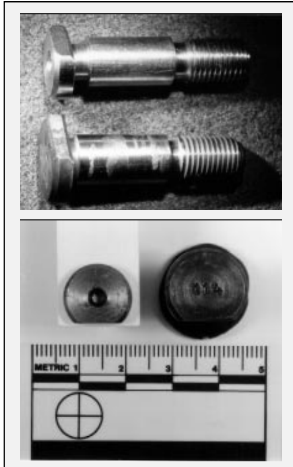
Fig. 2. The non-spec bolts: the upper bolt in the top photo; the bolt on the left in the lower photo.
