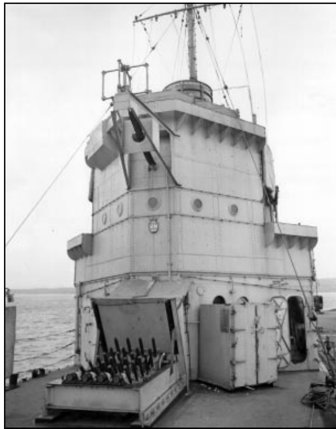
This 1944 view of the Hedgehog mounting on board the minesweeper HMCS Fort Francis shows just what a modest affair it was. (DND photo HS-0374-3, courtesy the Directorate of History and Heritage)
