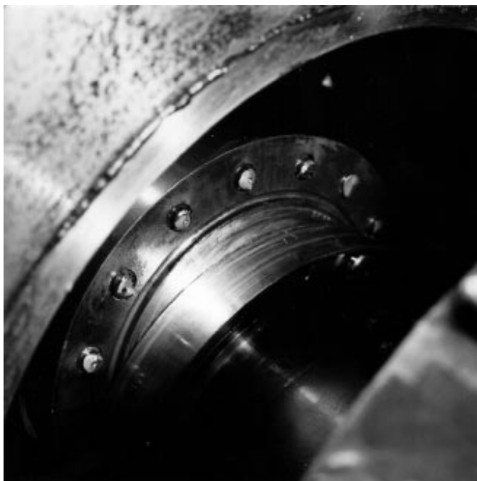
Fig. 3. Note the sheared off bolt heads on the connection between the auxiliary gearbox output shaft and the main gearbox cruise input shaft. (Base Esquimalt photo)
