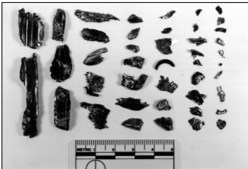
Fig. 6. Silent witness: this collection of bolt and nut material was recovered from the sump.
