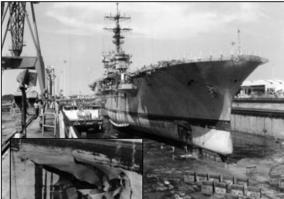
The amphibious assault ship USS Tripoli (LPH-10) lies in drydock in Bahrain after sustaining damage below the waterline from an Iraqi mine off Kuwait during the Gulf War in 1991. The ship was able to continue operations after damage control crews were able to stop the flooding. (USN photo by JO1 Joe Gawlowicz. Used with permission.)
