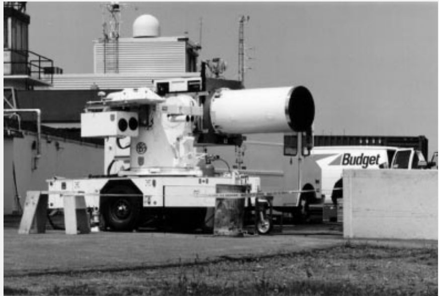
Defence Research Establishment Valcartier's trailer-mounted infrared imaging spectrometer has been used to measure IR signatures of Canadian warships. The imaging spectrometer produces a series of multidimensional graphed outputs of a ship's IR intensity mapped against different variables.
