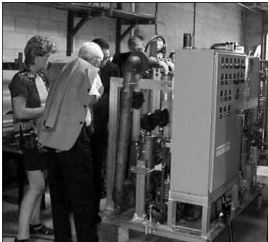
Workshop participants get a close look at the navy's new Hydromem™ Oily Water Separator in operation at Conor Pacific Environmental Technologies Inc.
