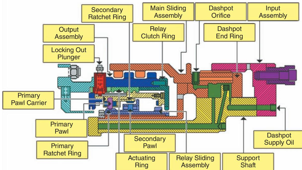
Figure 2. Simplified detail of the main components of the SSS clutch.
