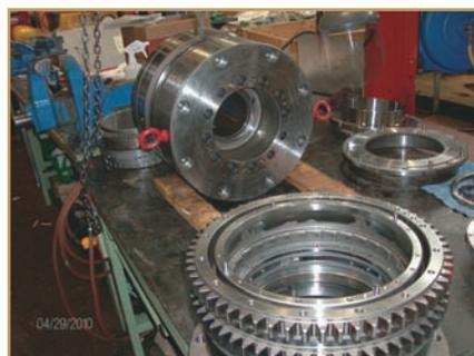
Step 9. The partially disassembled clutch sits on the bench for visual inspection at FMF *Cape Scott*.
