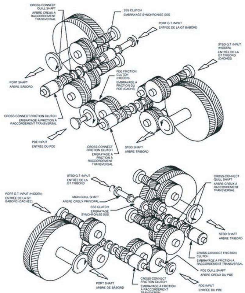
Figure 1. The gear component relationship on board the Halifax-class frigates<sup>2</sup>.
