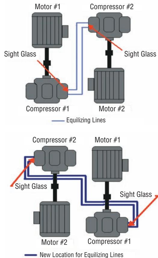
Figure 4. Compressor-motor assemblies before and after reconfiguration
