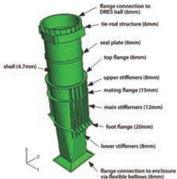
Figure 2. Original design of the original (existing) uptake with boundary conditions.
