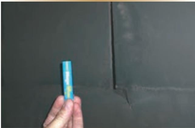
Figure 1a. It will take more than a cosmetic repair to close this thermally induced crack along a forward main vertical stiffener in HMCS *Montreal*'s starboard gas turbine uptake.
