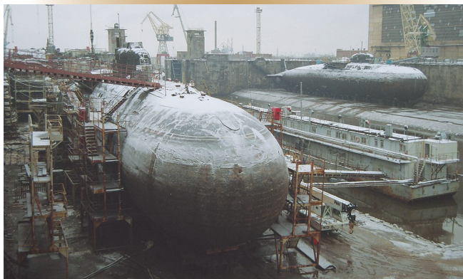
A Victor III SSN awaits dismantlement (left) at the Zvyozdochka Shipyard in Severodvinsk, and the same vessel 50-percent dismantled two months later (right).
