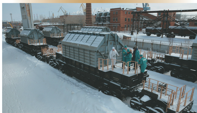
With the spent nuclear fuel assemblies safely stowed, a special train serves as temporary storage before making the long journey to deliver its radioactive cargo to the disposal facility at Mayak in the Urals.
