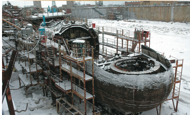
A Victor III SSN awaits dismantlement (left) at the Zvyozdochka Shipyard in Severodvinsk, and the same vessel 50-percent dismantled two months later (right).
