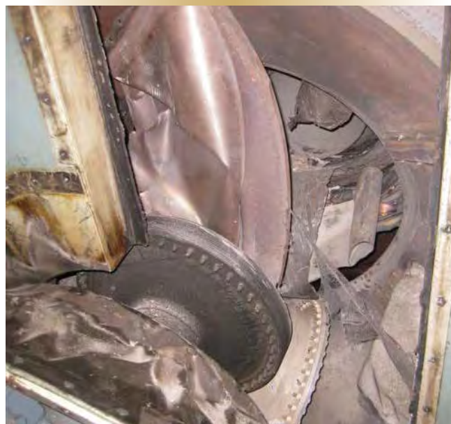
Figure 5 – What the exhaust duct (no. 1) and HSCS (no. 48) were supposed to look like – and what Toronto's engineering staff found.
