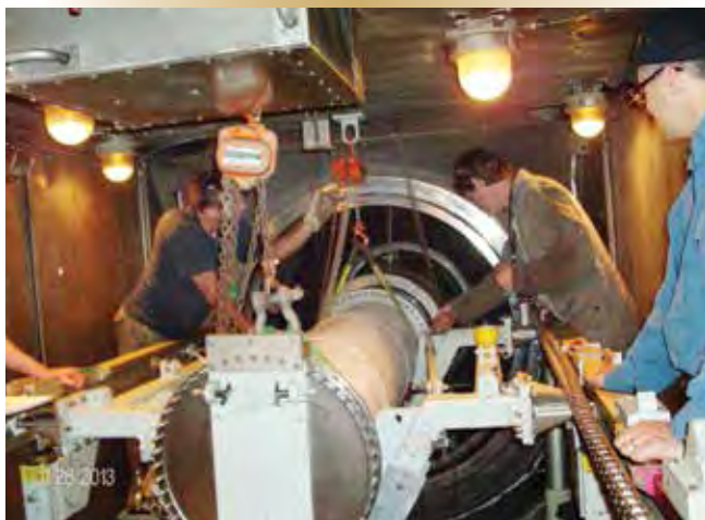
Figure 12 – FMFCS rigger Joshua Gordon, plater Ricardo Green and HMCS Toronto 's PO1 Steve Beaulieu install the new high-speed coupling shaft.
