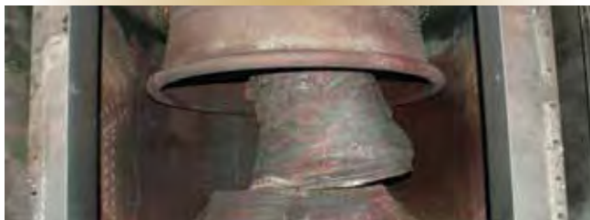
Figure 4 – Looking down into the engine exhaust duct of the enclosure, ship's staff get their first view of the damage to the HSCS.
