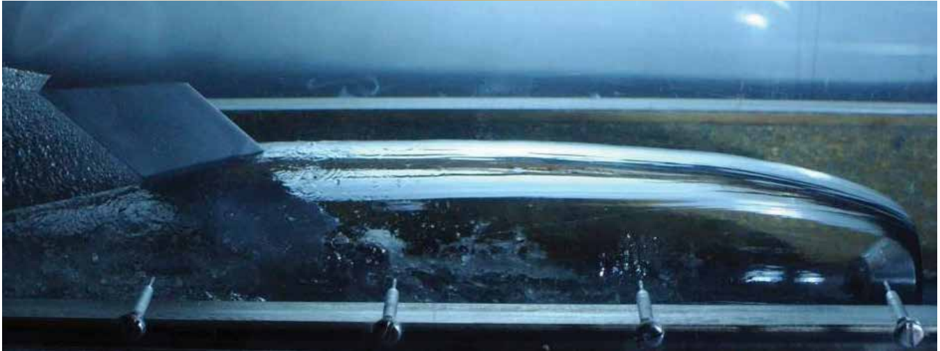
Figure 3 – Controlling a supercavitating body is a complex dance between aerodynamics within the gas cavity and hydrodynamics in the sea surrounding the bubble. (Source: http://cav.safll.umn.edu/gallery.htm )
