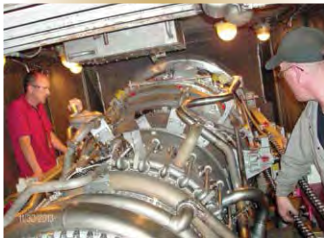
Figure 13 – GE field service rep Del Rogers (left) and FMFCS navy GT tech LS John Alford mate the gas generator to the power turbine. The ship went on to conduct sea trials days ahead of schedule.
