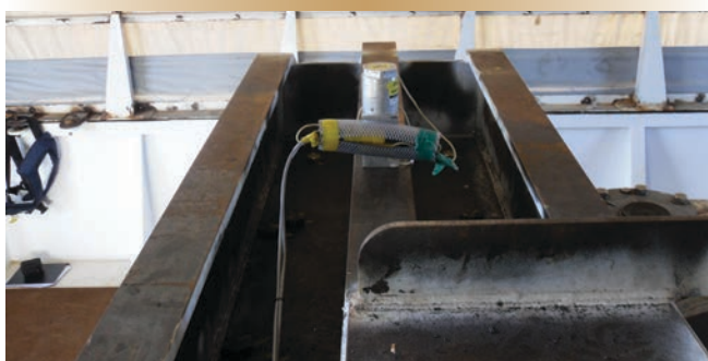
Figure 5. Accelerometers attached to the crane support (left) and to the heavy steel platform of the DSF II deck simulator fixture returned data that verified the proper execution of the heavyweight shock test trials, which were deemed a success.
