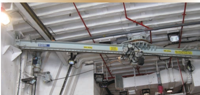
Figure 1. The MHP crane as fitted in HMCS Montréal 's hangar. The ship was the designated frigate for the Maritime Helicopter Project acceptance trials.
