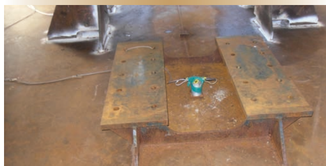
Figure 5. Accelerometers attached to the crane support (left) and to the heavy steel platform of the DSF II deck simulator fixture returned data that verified the proper execution of the heavyweight shock test trials, which were deemed a success.
