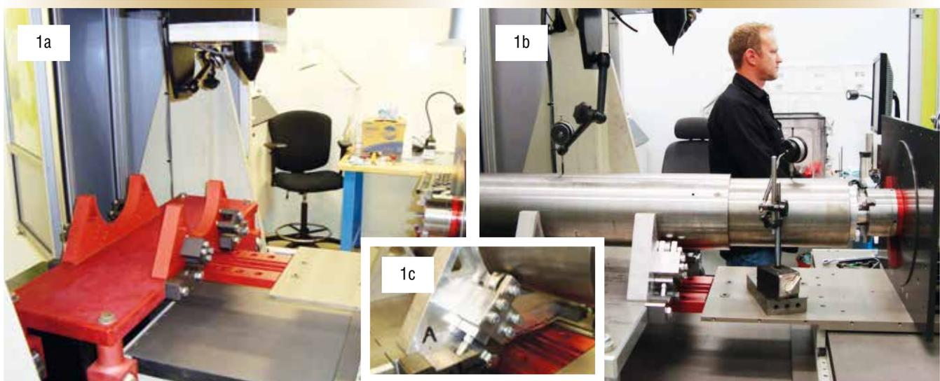
Figure 1a. The shaft LAM jig after application of an anodized protective coating. Figure 1b. The (uncoated) shaft LAM jig with a shaft in-situ to be worked on. Figure 1c. Adjustable rollers permit work to be done on varying shaft diameters.
