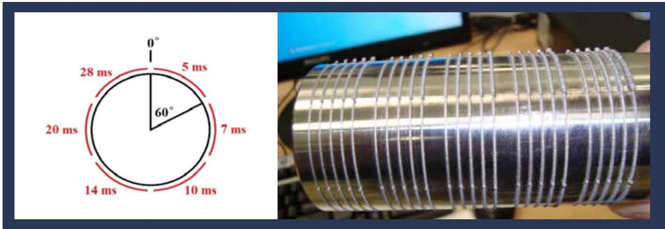
Figure 2. Test Specimen for Parameter Development: The test bar has 25 test strips arranged in five sets of five along the bar. The dial, showing an end-on view of the test bar, illustrates how the pulse duration in milliseconds (ms) was changed at 60-degree intervals around each test strip (for a total of 150 test spots along the bar).
