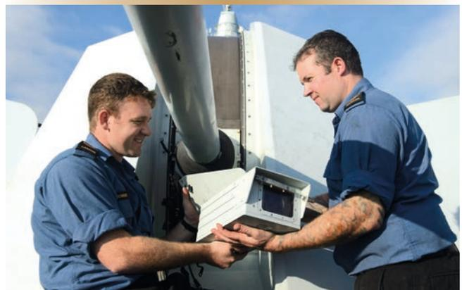
Careful preparation was the key to success. WENG technicians remove the rammer (left) and gun camera (right).
