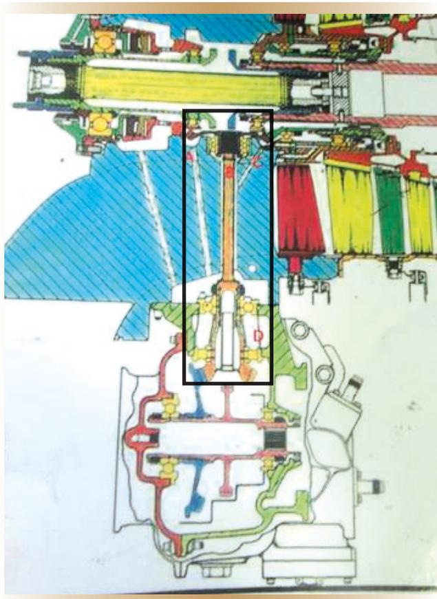
Figure 1. Location of tower shaft between the accessory gearbox and the engine shaft.
