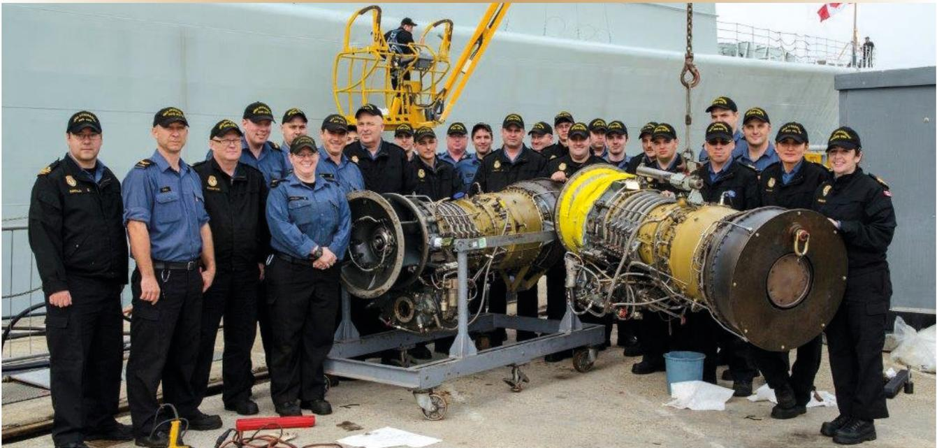
On Sept. 28 2015, while deployed in preparation for exercise Joint Warrior off the west coast of Europe, Her Majesty's Canadian Ship *Athabaskan* (DDG-282) experienced a failure of the starboard cruise gas-turbine engine. This article describes the failure and resultant engine change-out in a foreign port.
