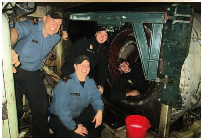
Figure 3. A swivel arm was rigged to manoeuvre the engine in the confined machinery space.
