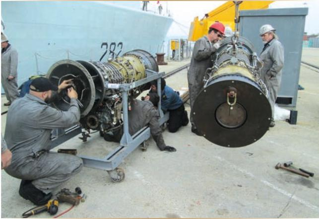
Figure 6. Exchanging connections from the old engine to the new.
