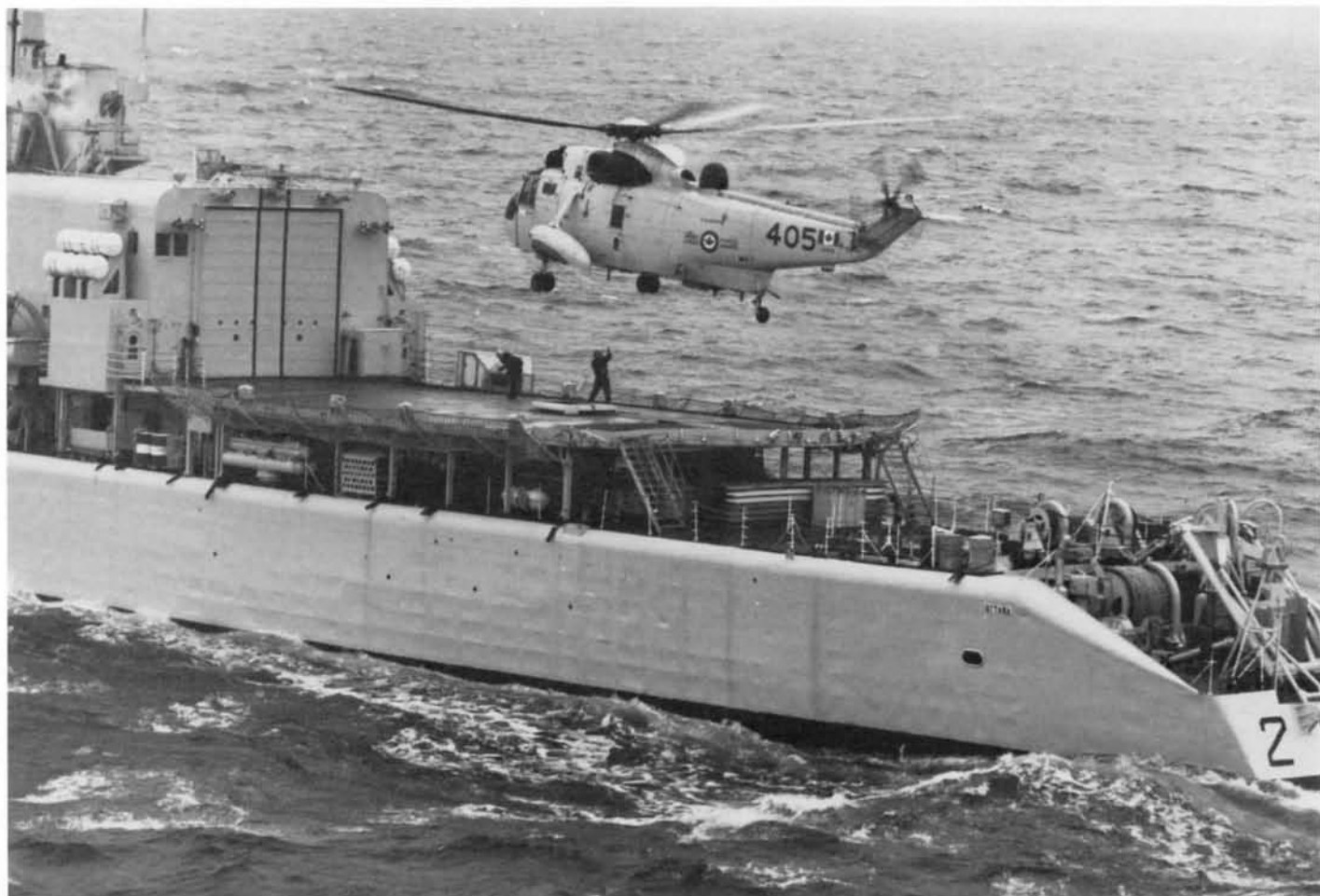
As the helicopter hovers over the flight-deck, the constant-tension cable is manually connected to the aircraft's messenger cable to be winched up.
