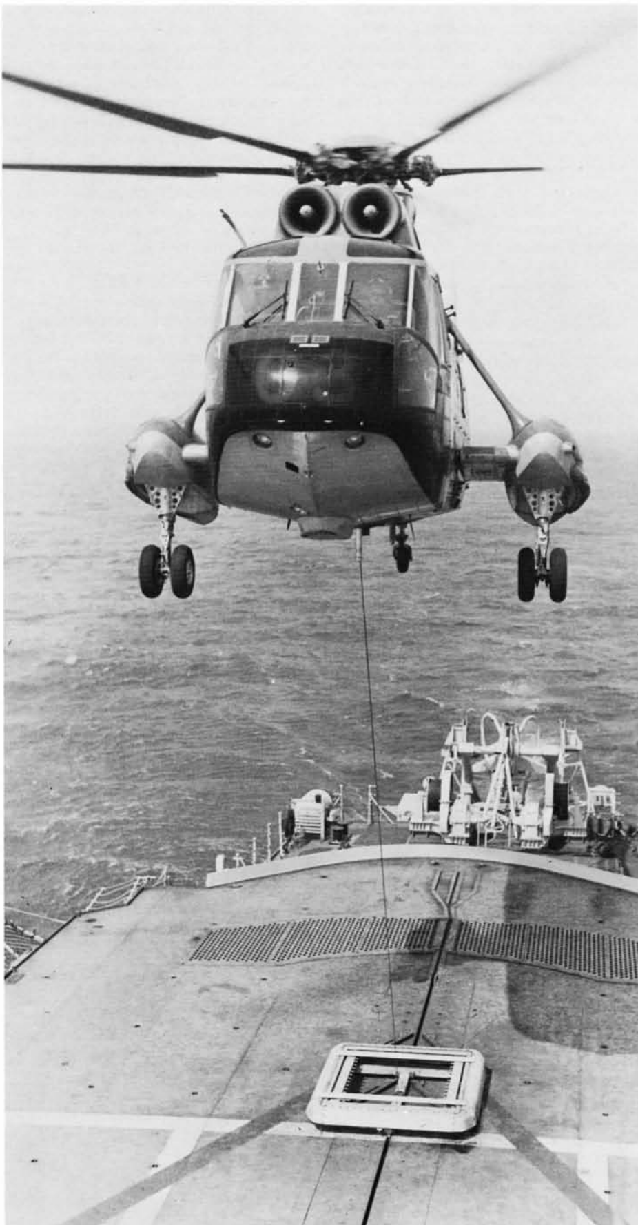
The pilot, still in control, flies the Sea King down to the deck with the assistance of the constant-tension hauldown cable. Once on the deck, the helicopter main probe is trapped in the jaws of the RSD by the Landing Signal Officer.
