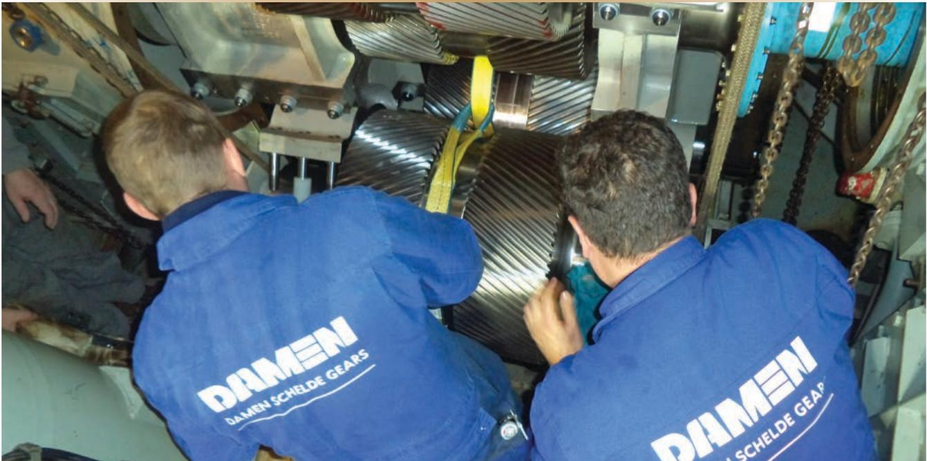
Figure 8. Idler gear being installed in the gearbox.
