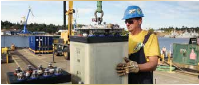
Each 550-kg cell battery acts as ballast in providing critical stability for the submarine.
