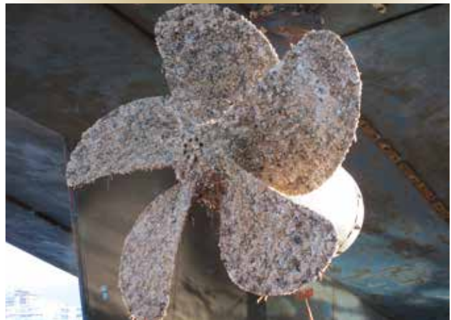
Figure 1. A fouled propeller of a vessel that sat alongside for 18 months in Victoria, BC. The extensive biofouling required removal by mechanical means, increasing the risk of propeller damage.
