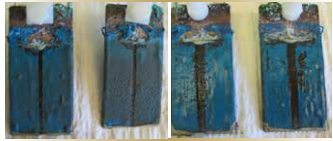
Figure 4. Front (left) and back (right) of cathodically-protected antifouling specimens after 18 months.
