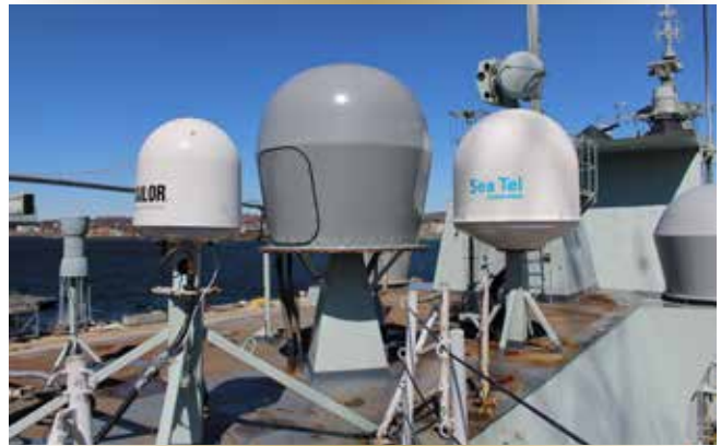
Figure 3. The AN/USC-69 SATCOM antenna (grey radome) has a nearly 245-degree unobstructed line of sight from its position on a frigate's hangar top.
