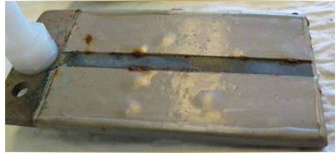
Figure 5. Epoxy specimens after 18 months of immersion, showing significant blistering at numerous locations.
