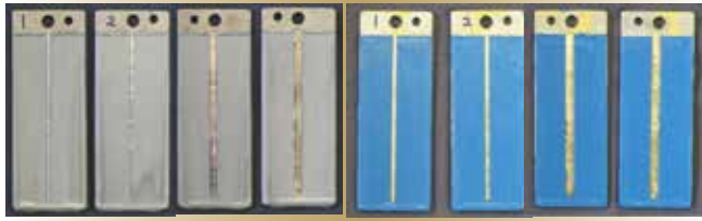
Figure 2. Front and back of epoxy-coated (left) and antifouling-coated (right) specimens after an intentional defect had been milled on both sides, and prior to immersion.
