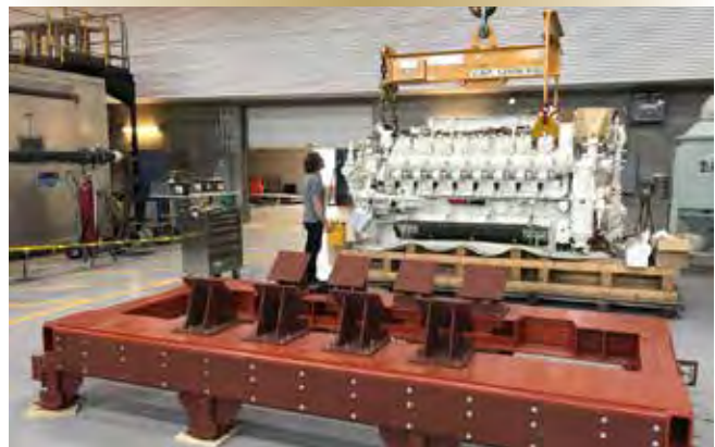
NETE Task Leader Carl Chamberland prepares to verify the installation of a PAXMAN engine on an engine cradle in the test cell.
