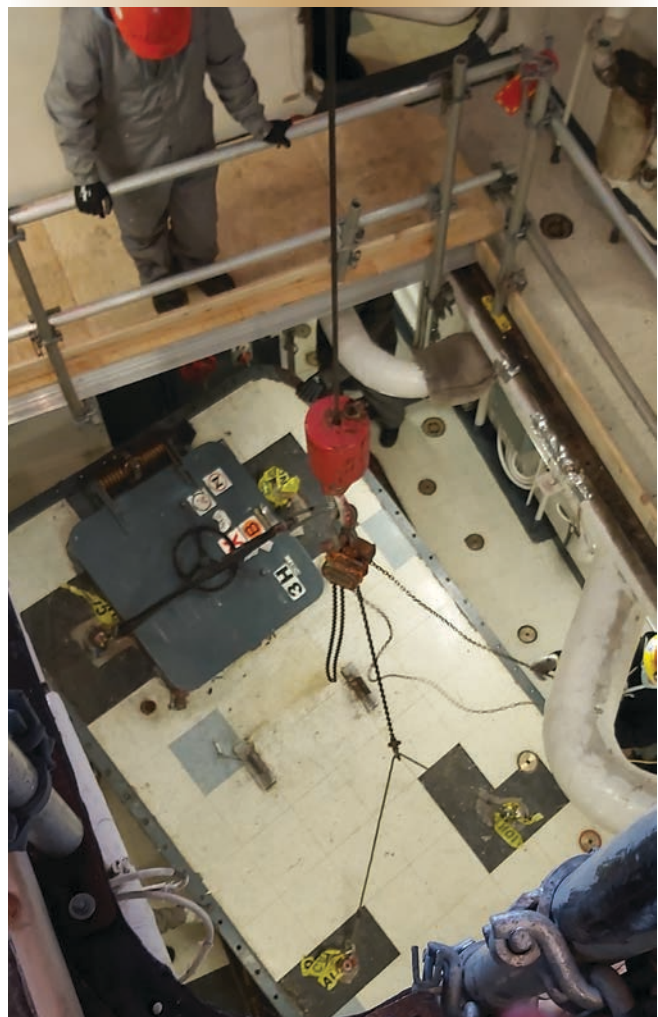
Figure 1. FMFCS personnel remove the soft patch into HMCS Ville de Québec 's after auxiliary machinery room (AAMR).
