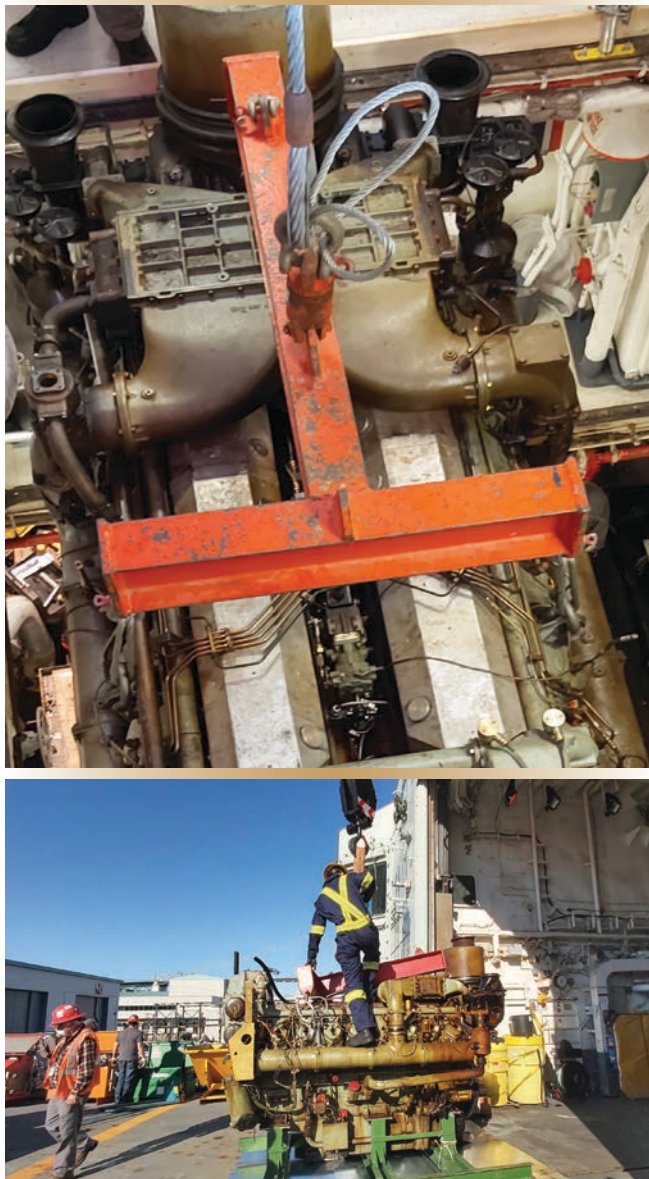
Figure 2a and b. A legacy MWM 602 engine is rigged and ready to be lifted out of the AAMR, and then craned ashore.
