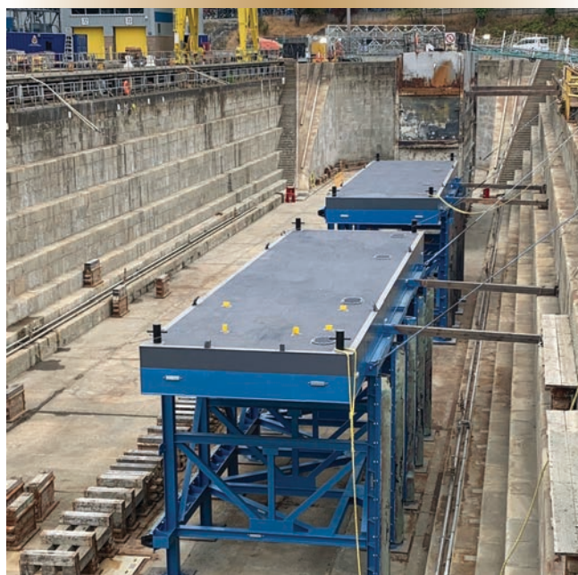
Figure 1. These two U.S. Navy submarine camel fender barges, on semi-permanent loan to the RCN, were completely refurbished and returned to service by Fleet Maintenance Facility Cape Breton in Esquimalt, BC.
